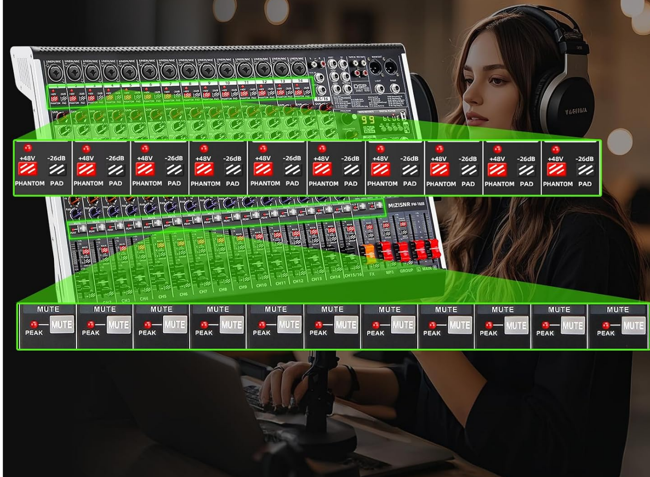
Image: Individual +48V Phantom Power and PAD switches for each channel, supporting various microphones.
