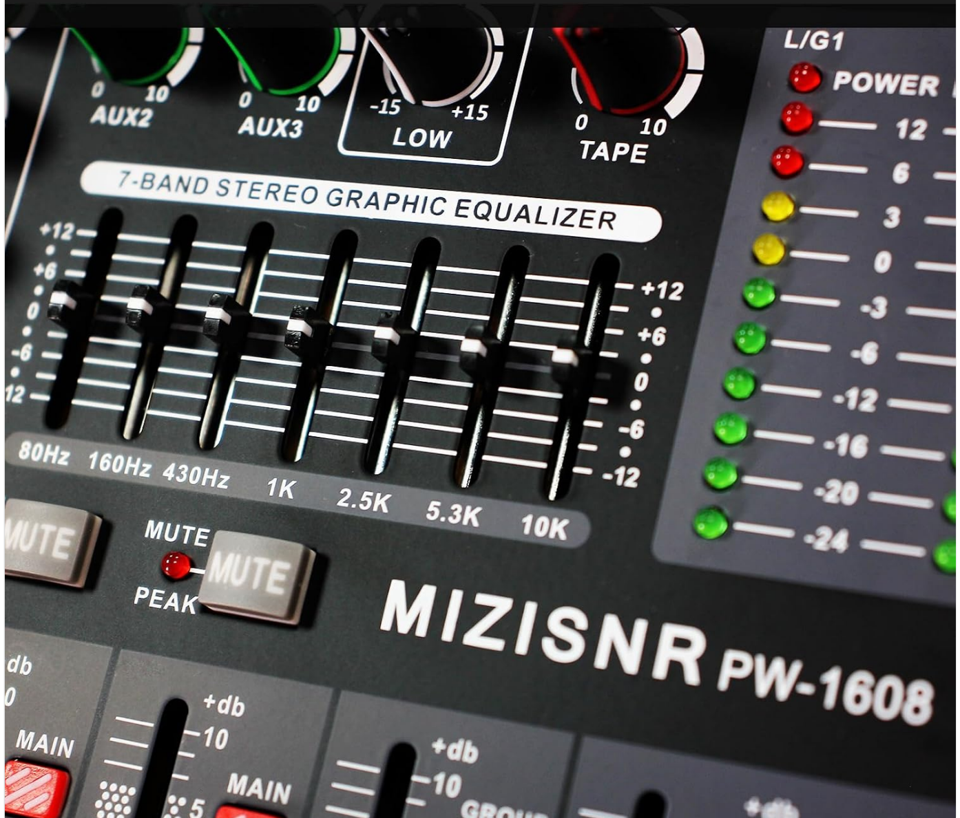
Image: The 7-band stereo graphic equalizer for precise main output tone control.
