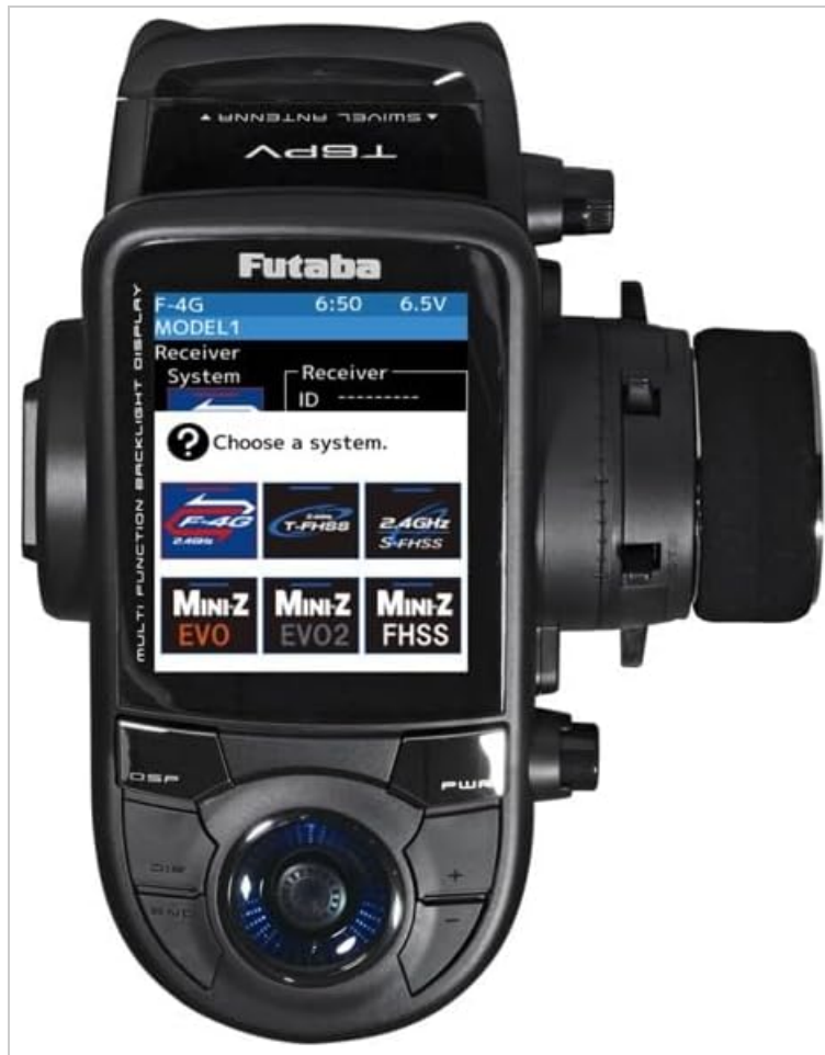
Image 5: The Futaba T6PV Transmitter's display showing the 'Receiver System' selection screen. Various compatible systems like F-4G, T-FHSS, S-FHSS, MINI-Z EVO, MINI-Z EVO2, and MINI-Z FHSS are presented as selectable options.
