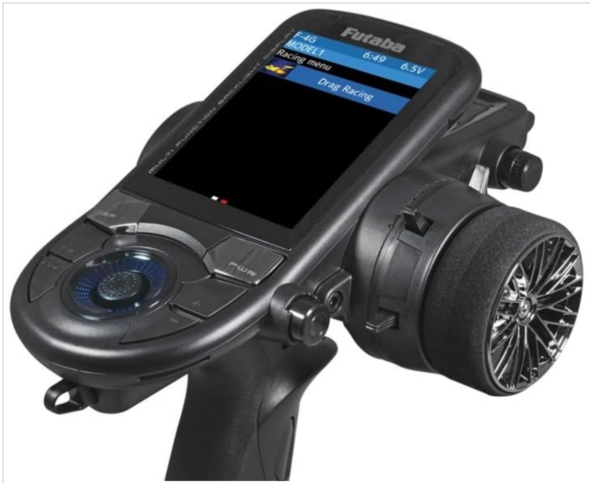
Image 6: The Futaba T6PV Transmitter's display showing a 'Racing menu' with 'Drag Racing' selected. This illustrates the specialized menus available for different RC disciplines and advanced tuning options.
