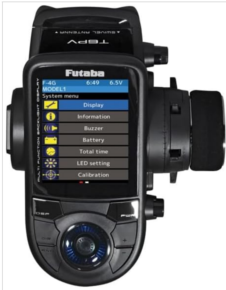
Image 4: The Futaba T6PV Transmitter's color LCD displaying the 'System menu'. Options visible include Display, Information, Buzzer, Battery, Total time, LED setting, and Calibration, demonstrating the user interface.
