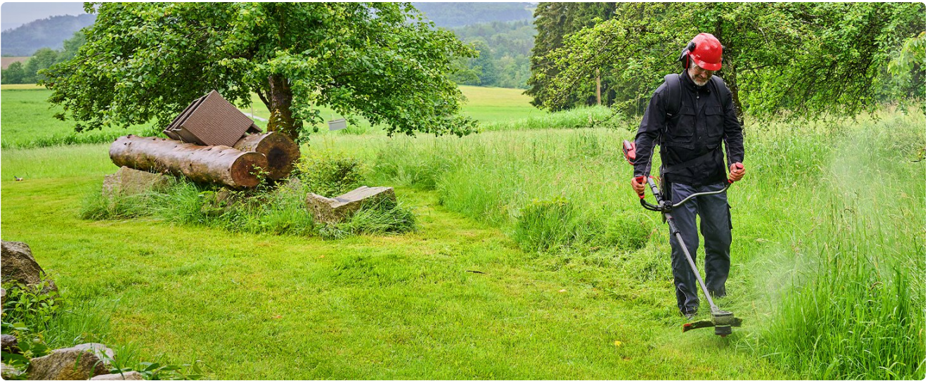
Figure 5.2: Maintain a comfortable and stable posture while operating, utilizing the backpack harness for support.
