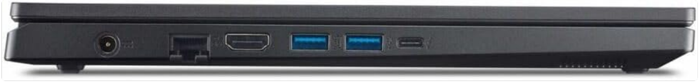
Figure 2: Left side ports including power, Ethernet, HDMI, USB-A, and USB-C.
