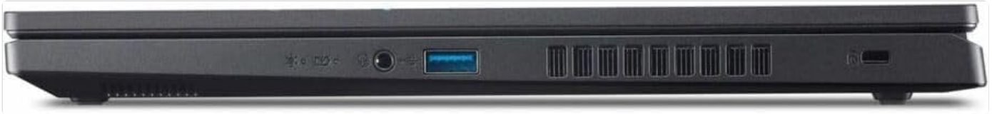
Figure 3: Right side ports including USB-A and headphone jack.
