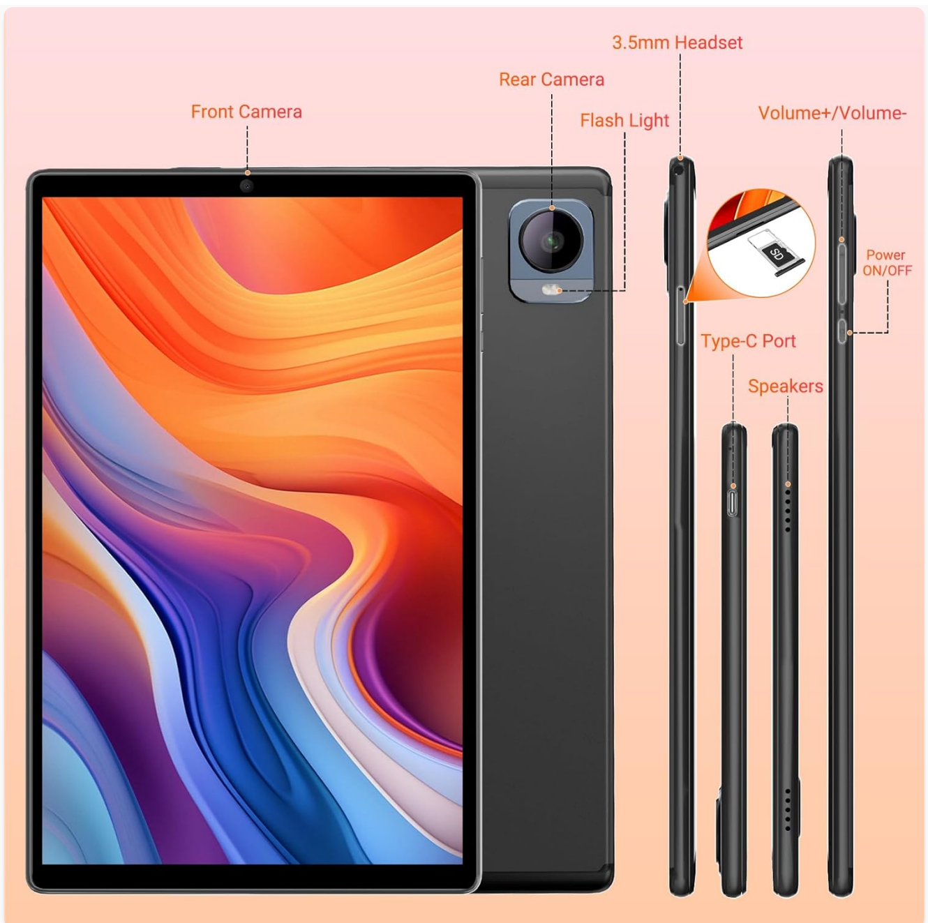
Image 2.2: Diagram showing the location of the front camera, rear camera, flash light, 3.5mm headset jack, volume buttons, Power ON/OFF button, Type-C port, speakers, and the SIM/SD card slot on the TIGERFU P107 tablet.
