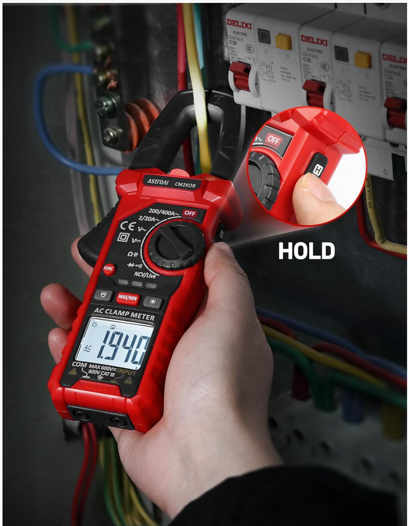
Figure 5.7: Activating the HOLD function to retain a measurement on the display.
