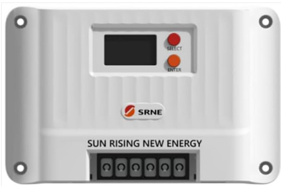
Figure 1.1: Front view of the SRNE Shiner2460 MPPT Solar Charge Controller, showing the display, 'SELECT' and 'ENTER' buttons, SRNE logo, and terminal block.
