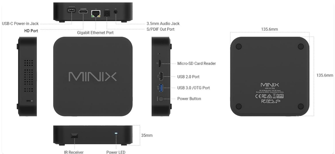
Figure 4: Detailed diagram of MINIX U8K-Ultra ports and dimensions.
