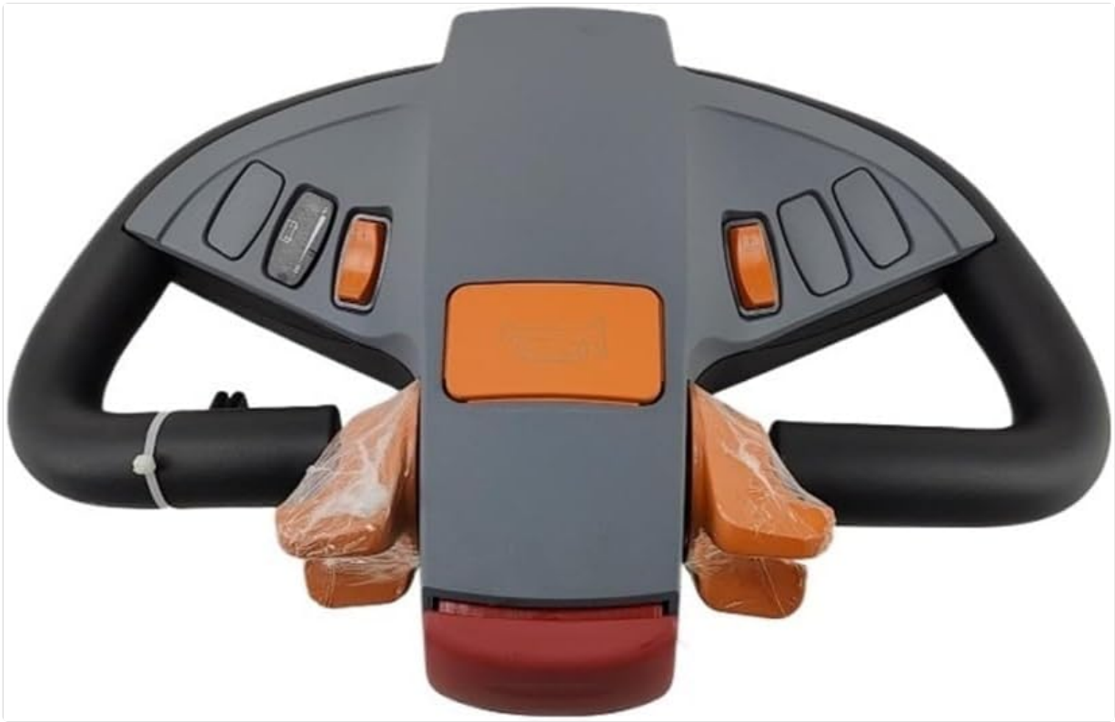
A top-down view of the handle, highlighting the central orange horn button, two smaller orange buttons, and the overall ergonomic design. This perspective provides a clear view of the button arrangement.
