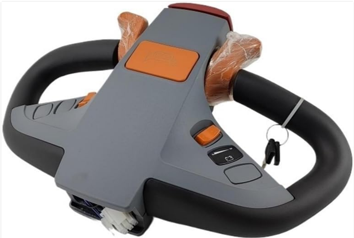
Another angled view of the handle, revealing the wiring harness at the base, indicating its readiness for electrical connection. This image shows the necessary connections for integration into the forklift's electrical system.
