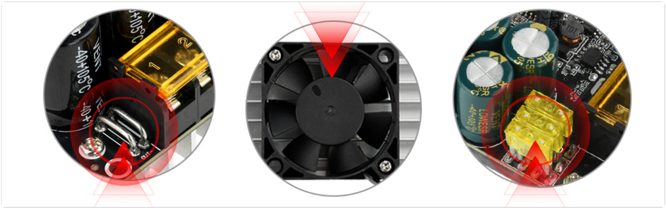
Figure 3.4: Detailed close-up shots of critical components: the replaceable fuses for overcurrent protection, the cooling fan for heat dissipation, and the large inductor coil, which is central to the boost conversion process.
