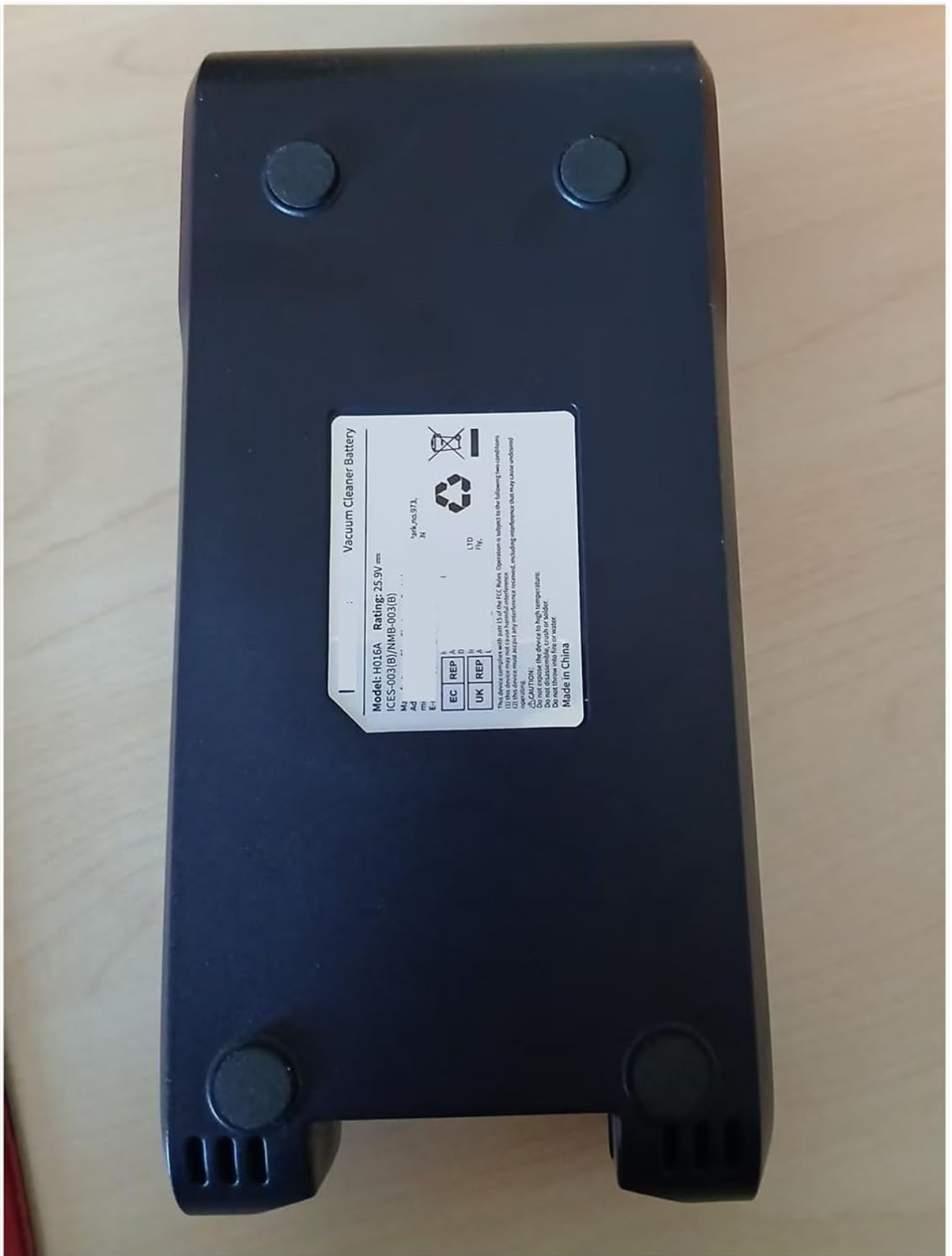
Figure 4: Bottom view of the H015R battery pack, highlighting the four rubber feet for stability and the electrical connection interface. This interface connects the battery to the vacuum cleaner.
