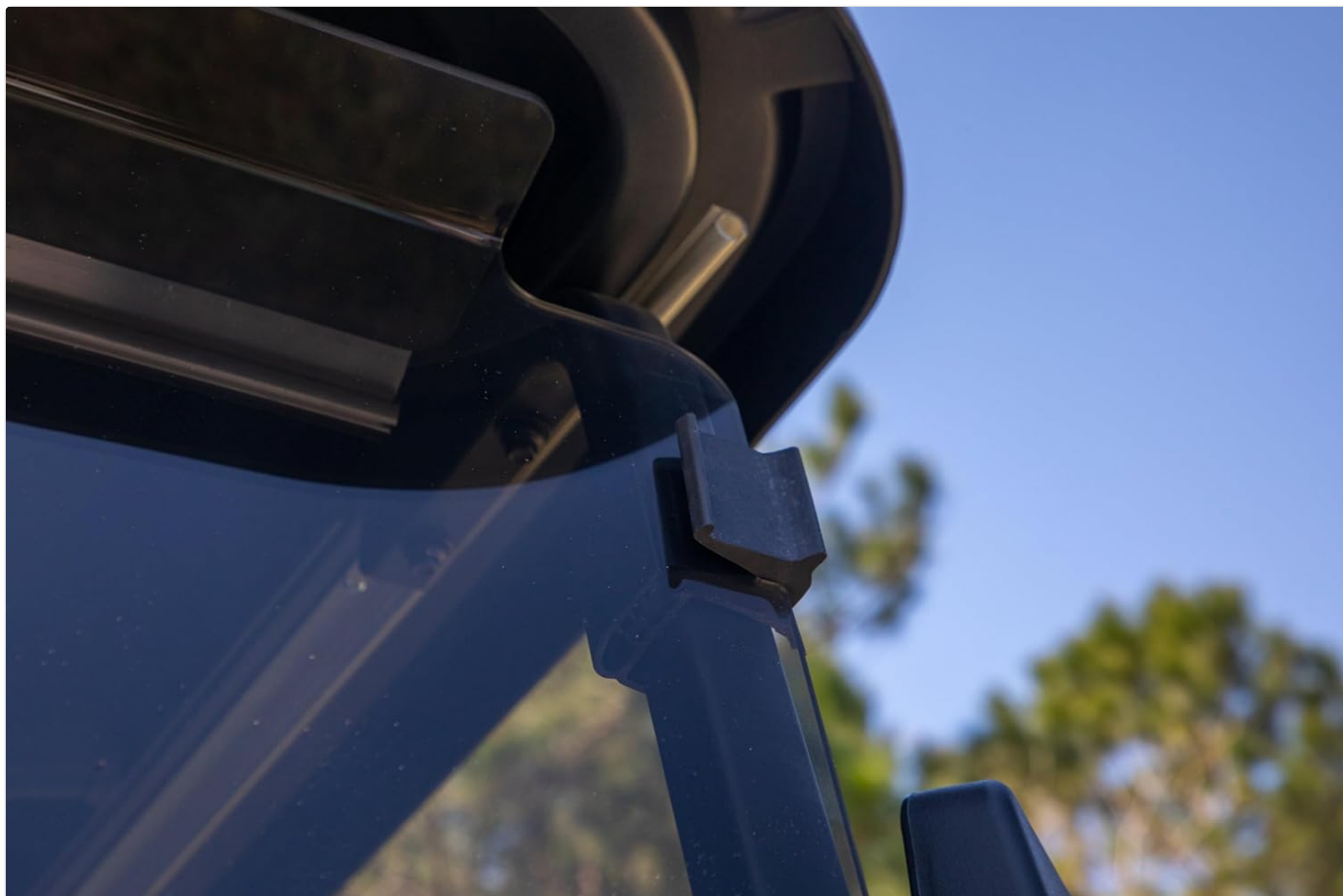
Figure 3.2.2: Detail of the top mounting clip.
