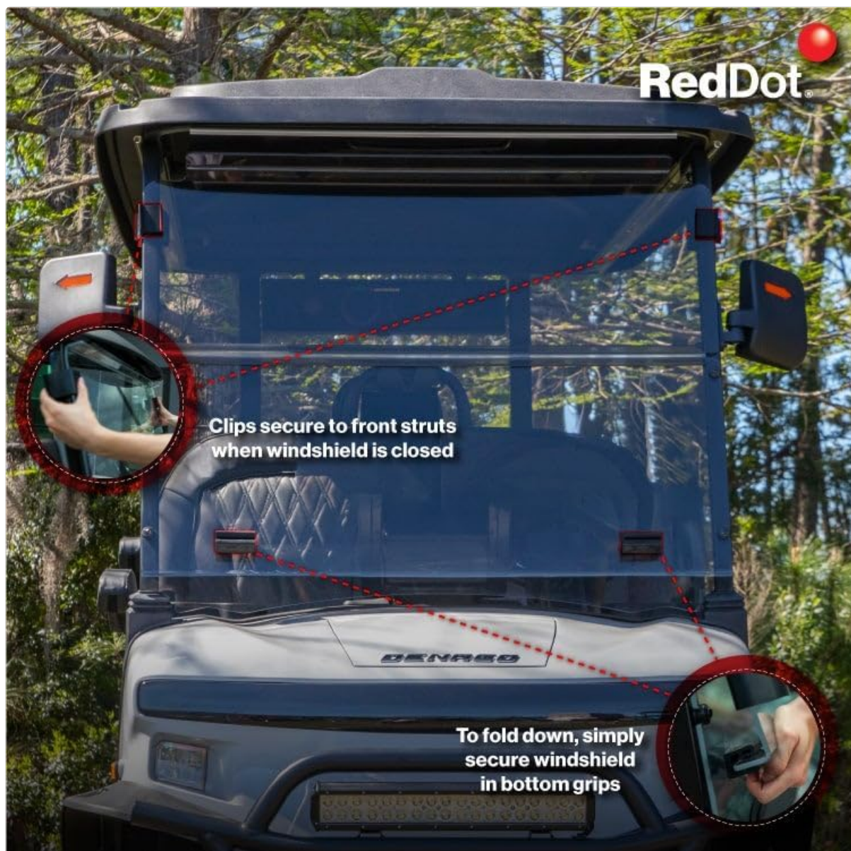
Figure 4.2.1: Demonstrating the folding and securing mechanism.
