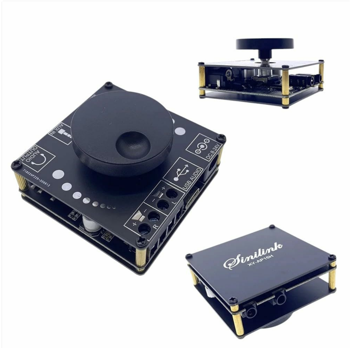
Image 1: Front view of the Sinilink XY-AP15H amplifier board, showing the central volume knob, USB audio input, DC power input (8-24V), AUX input, and speaker output terminals. The board is black with gold standoffs.
