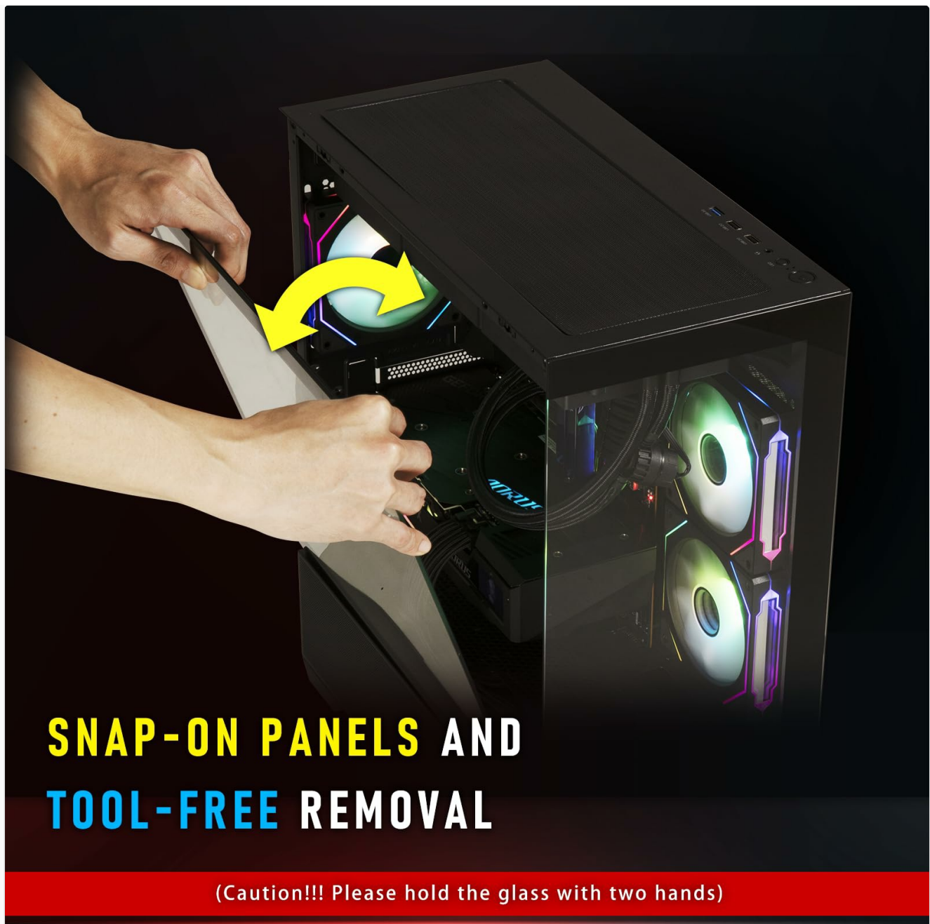
Figure 4: Removing the side panel. Always handle tempered glass with care, using both hands.
