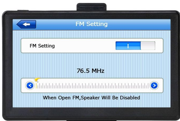
Figure 6: Instructions for setting up the FM Transmitter, demonstrating how to match the Sat Nav's frequency with the car's FM radio.
