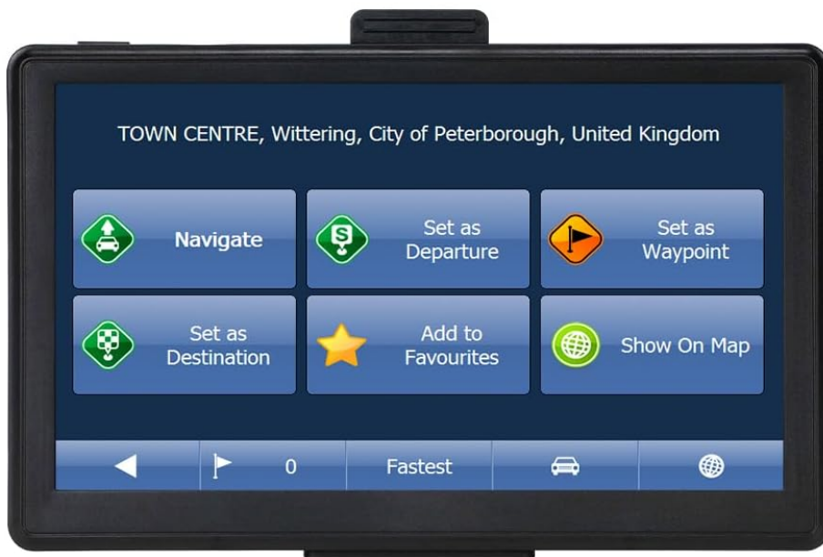
Figure 3: Main menu interface of the OHREX T76 Sat Nav, showing options like Navigate, Set as Departure, Set as Waypoint, and POI search.
