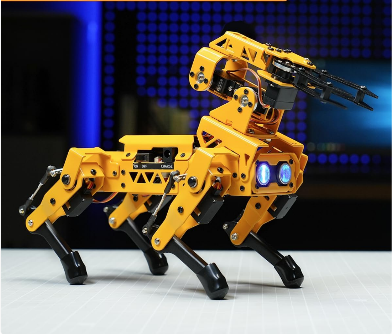
Image 3.1: MechDog Pro with the 3DOF robotic arm attached, ready for gripping and handling tasks.
