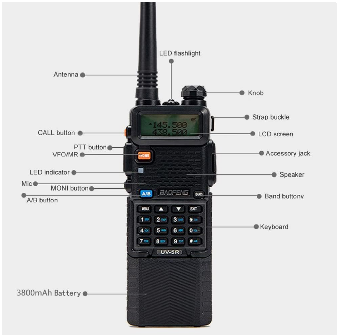
Detailed diagram identifying all external components of the UV-5R radio.
