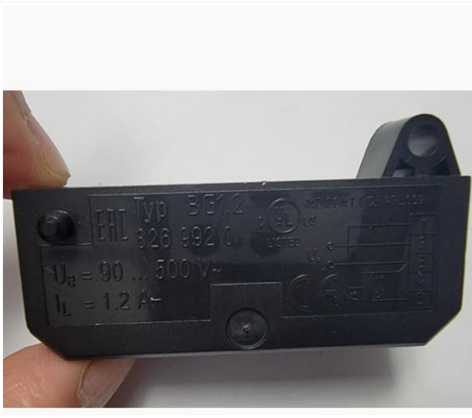
Figure 3.1: ZHRCLY BG1.2 Rectifier Module. This image shows the compact design of the BG1.2 module, typically used for converting AC to DC for motor brake applications.
