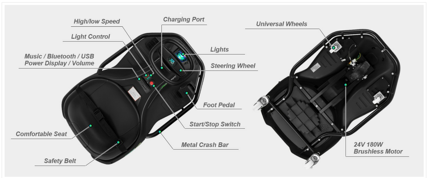
Image: Labeled diagram highlighting various parts of the drift car, such as the steering wheel, foot pedal, charging port, and safety belt.
