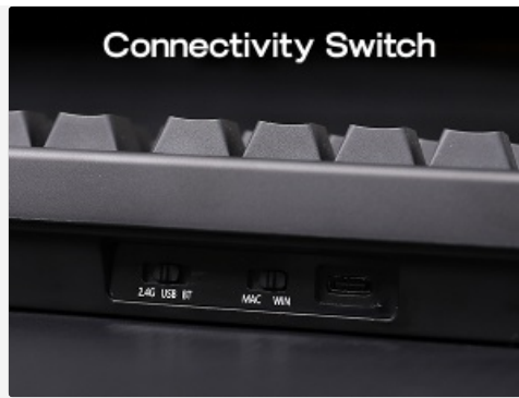
Figure 3: Connectivity and OS Mode Switches
