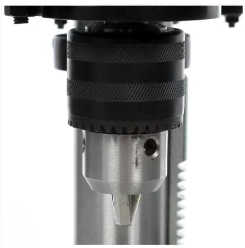
Figure 3: Drill Press Chuck. This image provides a close-up view of the drill chuck, where drill bits are inserted and secured. It shows the knurled grip for tightening and loosening the chuck jaws.
