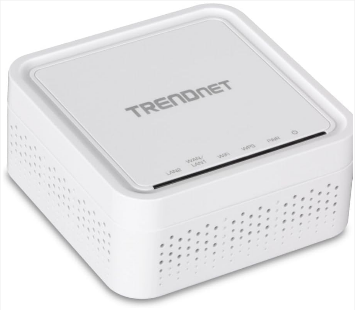
Image: The TRENDnet TEW-832MDR EasyMesh Node. This white, rectangular device features the "TRENDnet" logo on its top surface. Along the front edge of the top panel, there are indicator lights and labels for LAN2, WAN/LAN1, WiFi, WPS, and PAIR, along with a power symbol. The sides of the device have ventilation holes.
