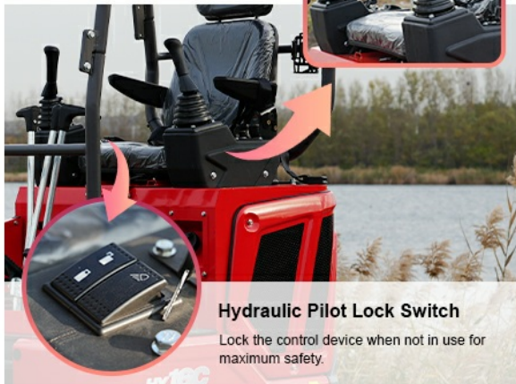
Figure 5.2: Visual representation of the Hydraulic Pilot Function and Swing Arm Function controls.
