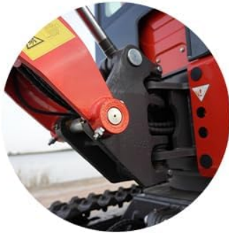
Figure 5.3: The excavator's swing arm function allows for precise positioning of the boom and bucket without repositioning the entire machine.
