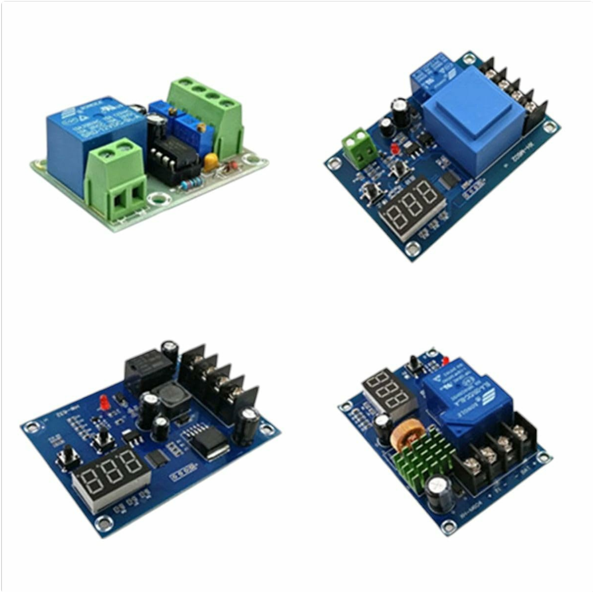
Figure 1: Assortment of ROXIFETA XH-M60x series battery protection board modules. These modules are designed for various battery management tasks, featuring different layouts and components depending on the specific model.
