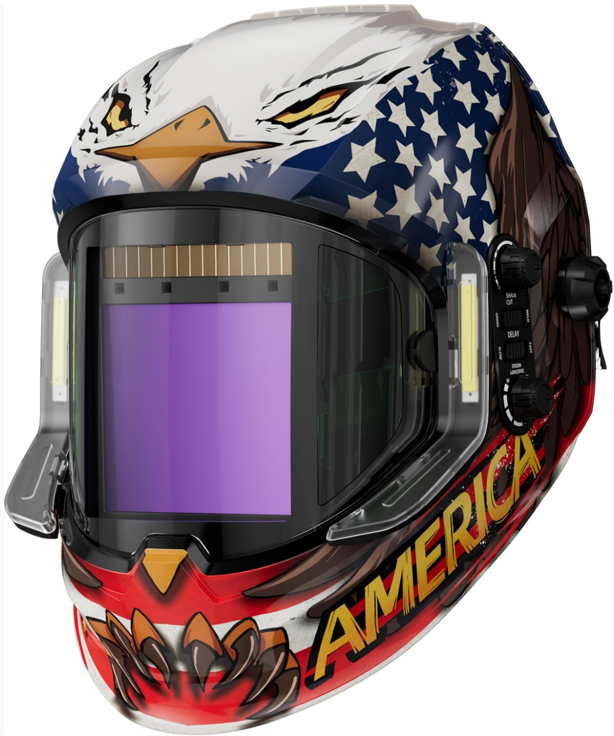
Figure 4.3: External Controls. The side of the helmet features rotary knobs for adjusting the delay time (how long the lens stays dark after the arc stops) and sensitivity (how easily the sensors detect an arc). A switch for Grind/Cut mode is also present.
