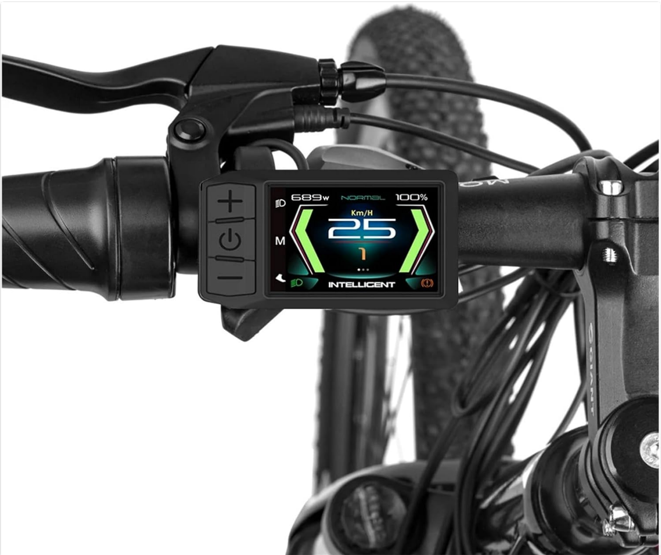
Image 4.1: The 600C-CAN display securely mounted on an e-bike handlebar, showing its position relative to other controls.
