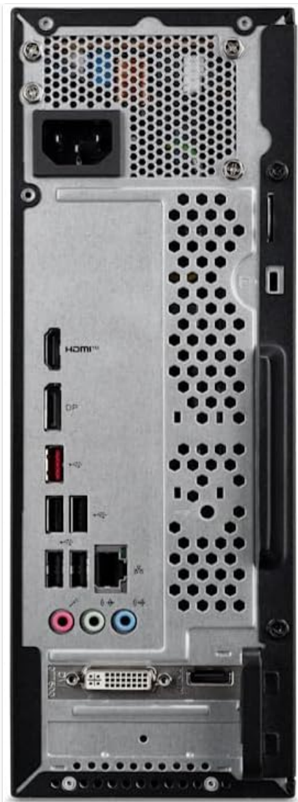
Image: Rear view of the Acer Aspire XC-1860 desktop tower, displaying various connectivity ports including HDMI, DisplayPort, USB, Ethernet, and audio jacks.
