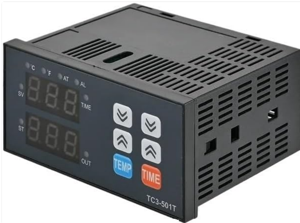
This image displays the front panel of the TC3-501T PID Temperature Controller. It features two digital displays for Set Value (SV) and Current Temperature (ST), along with indicator lights for output (OUT), alarm (AL), and auto-tuning (AT). Control buttons include up/down arrows for adjustment, and dedicated buttons for 'TEMP' and 'TIME' settings.
