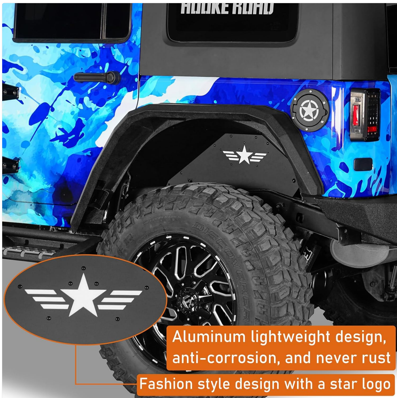
Image: A detailed view of the rear fender liner, emphasizing its lightweight aluminum design, anti-corrosion properties, and the stylish star logo.
