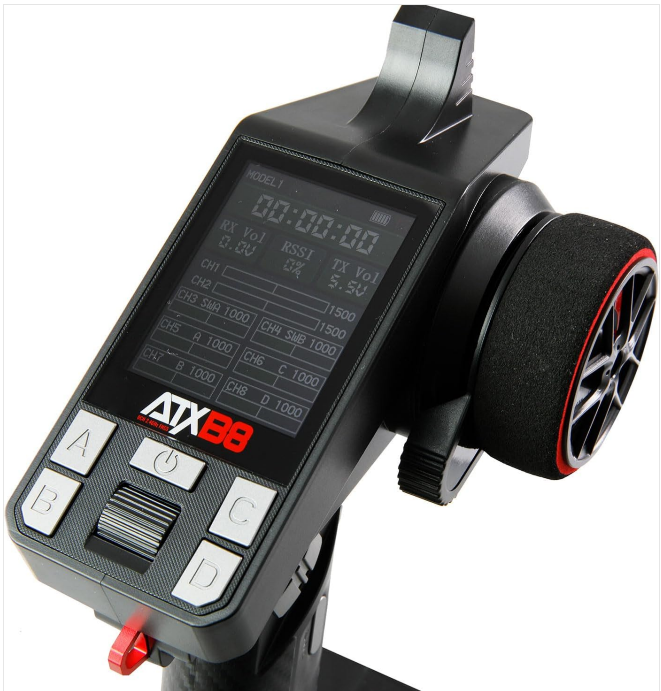
Figure 3: The ATXB8's color display showing channel and telemetry information.
