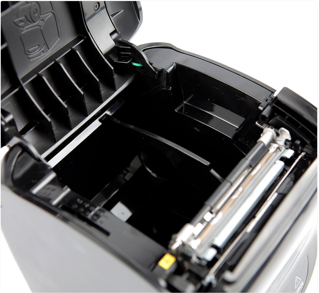
Figure 3: Printer paper loading mechanism.
