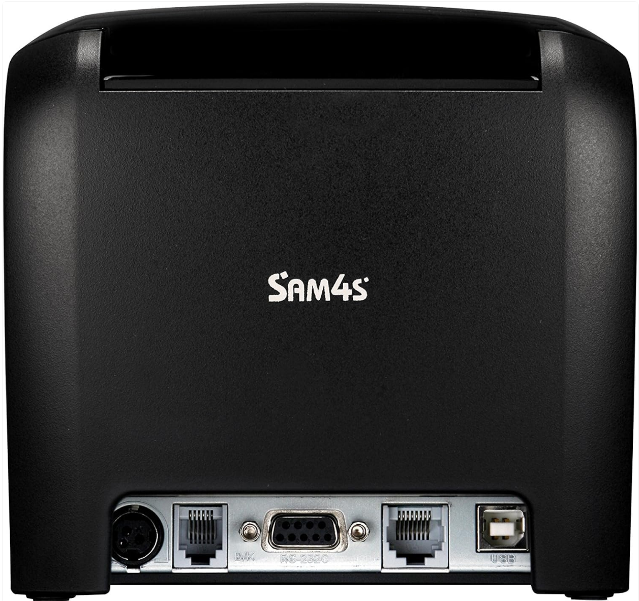
Figure 2: Printer rear view with connectivity ports.
