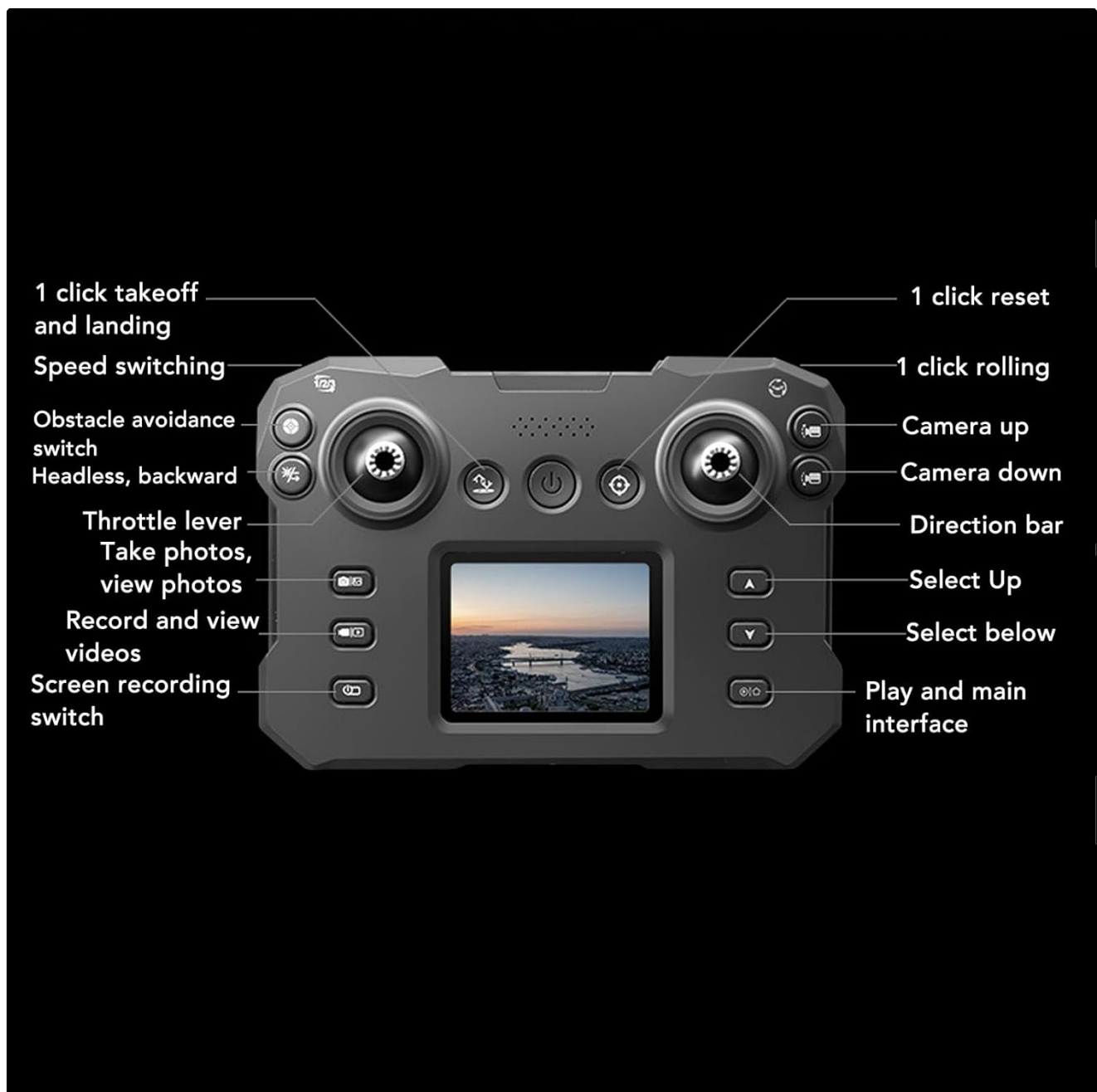
Image: Detailed diagram of the remote control, showing the function of each button and joystick, including 1-click takeoff/landing, speed switching, obstacle avoidance switch, headless mode, camera controls, and screen recording.
