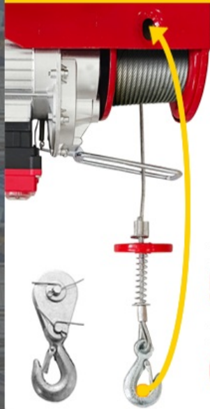
Image 6.1: Comparison of single-cable and double-cable lifting methods, illustrating how the pulley block doubles the lifting capacity while halving the speed and height.
