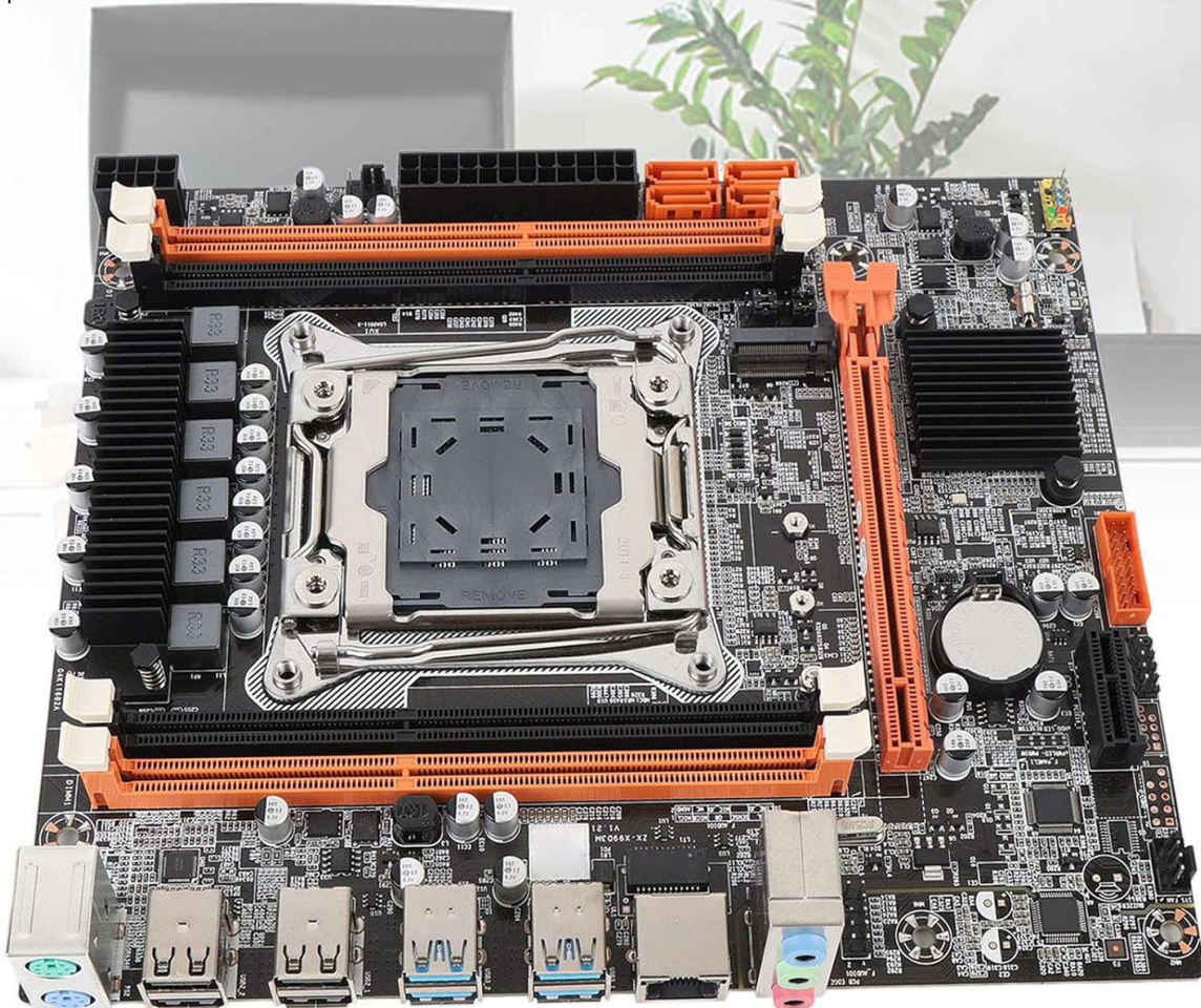
Image 4.1: Close-up of the LGA 2011-3 CPU socket. This image shows the socket where the processor is installed, emphasizing the retention mechanism.
