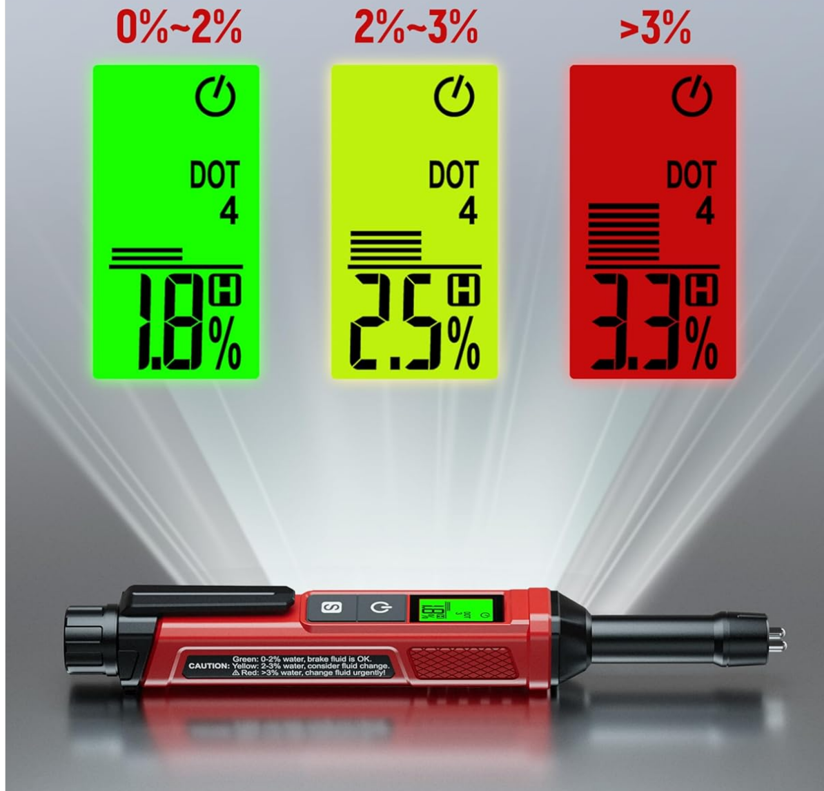
Image 5.4: KAIWEETS KVBF01 Brake Fluid Tester displaying 3 colors backlight. The image shows the tester's display changing color (green, yellow, red) based on the water content percentage, indicating the condition of the brake fluid.
