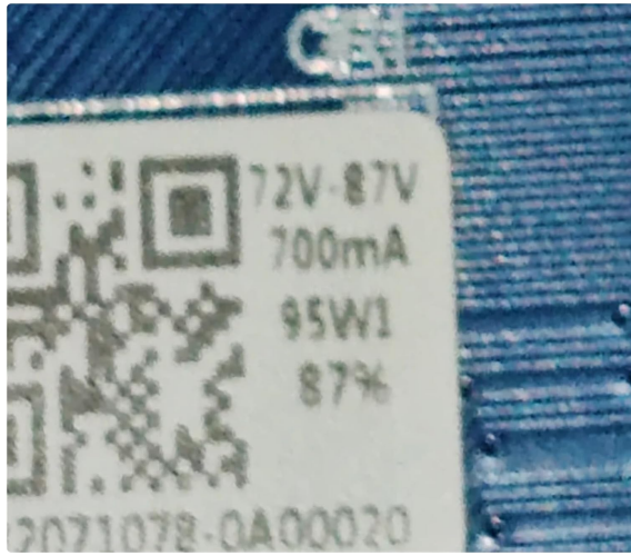
Image: Close-up of a label displaying a QR code and power specifications such as voltage (72V-87V), current (700mA), and wattage (95W1).
