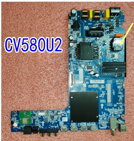
Image: YSVQHHDV TV Motherboard, model CV580U2, showing the main circuit board layout and components.
