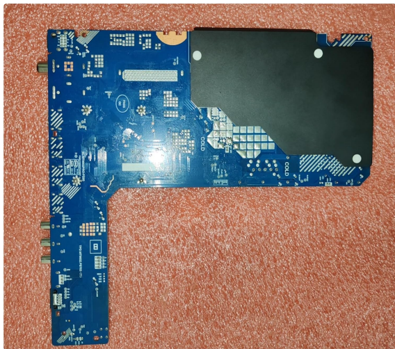
Image: Rear view of the TV motherboard, displaying the solder points and circuit traces on the underside.
