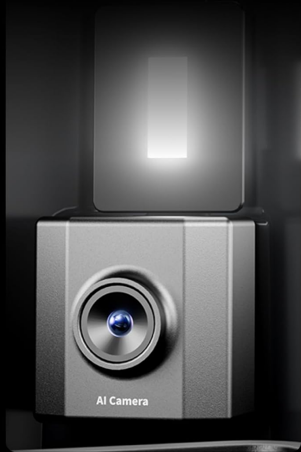
Image 4.3: The AI camera and lighting system for print monitoring.
