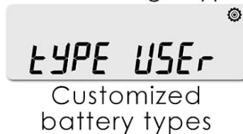
Image 4.1: Display showing selectable battery types (TYPE 01-08, USER) and corresponding selectable battery voltages (DC12V, 24V, 36V, 48V).
