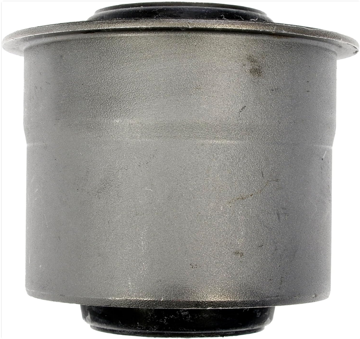
Image 4.1: Side view of the Dorman 533-958 Front Rearward Radius Arm Bushing. This perspective highlights the cylindrical body and the flared ends, which are critical for proper seating within the radius arm and vehicle frame.
