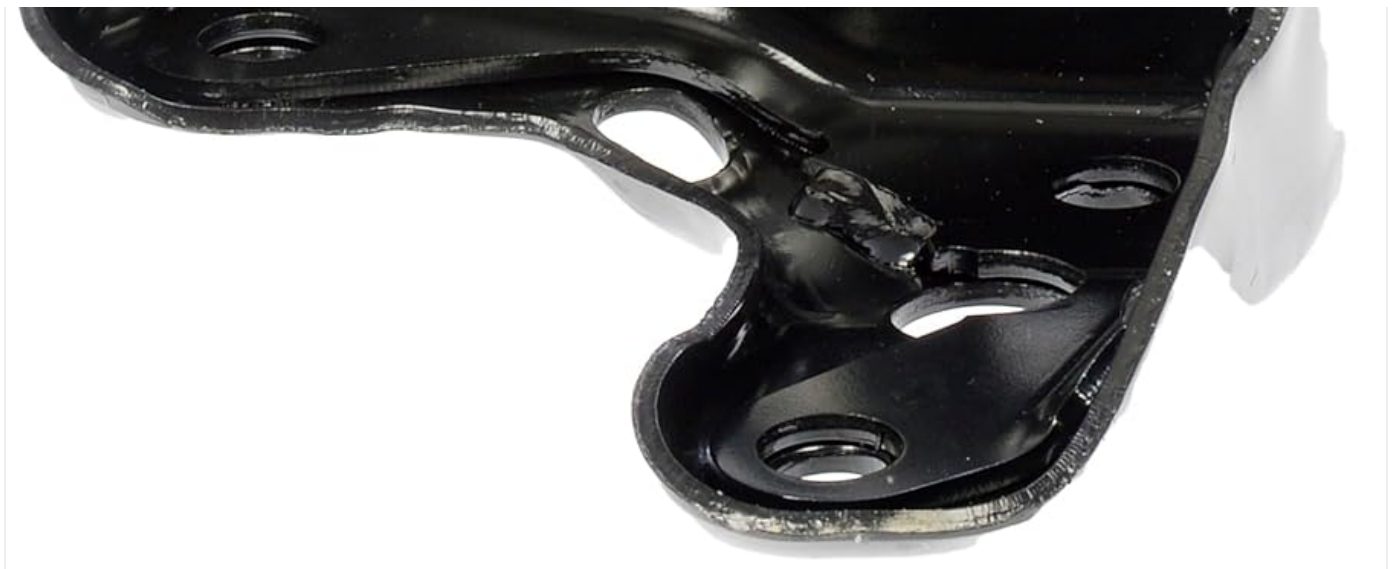
Figure 6.1: Detailed view of the Dorman 526-039 trailing arm's body, showing mounting points. Regular inspection of these areas is important for maintenance.
