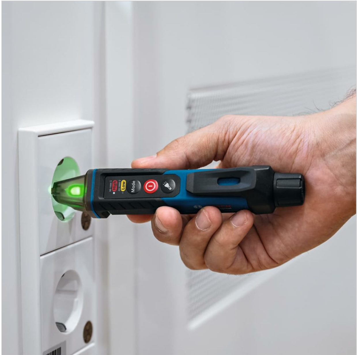
Figure 5: Using the Bosch GVD 1000-17 to detect voltage in a wall socket.
