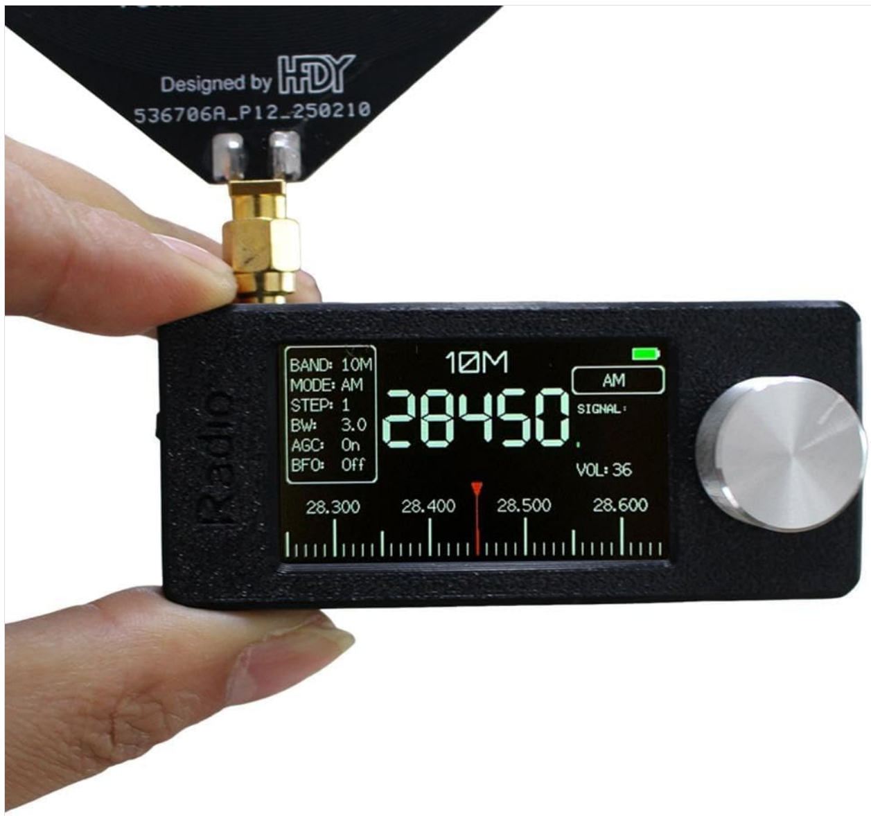
Image 3.2.2: The radio connected to the external loop antenna, which enhances reception across various bands.
