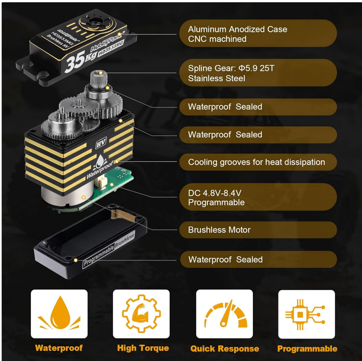
Image 4.2: Exploded view highlighting key features such as the aluminum anodized CNC machined case, stainless steel spline gear, waterproof seals, cooling grooves, programmable DC 4.8V-8.4V operation, and brushless motor.
