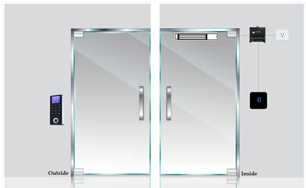
Figure 4.2.5: System Component Placement (Outside vs. Inside)
