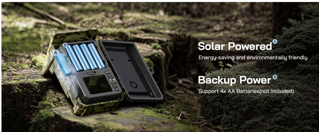
Figure 2.2: Internal Battery and AA Battery Slots. This image shows the camera's interior with the rechargeable lithium battery (A) and slots for optional AA backup batteries (B).
