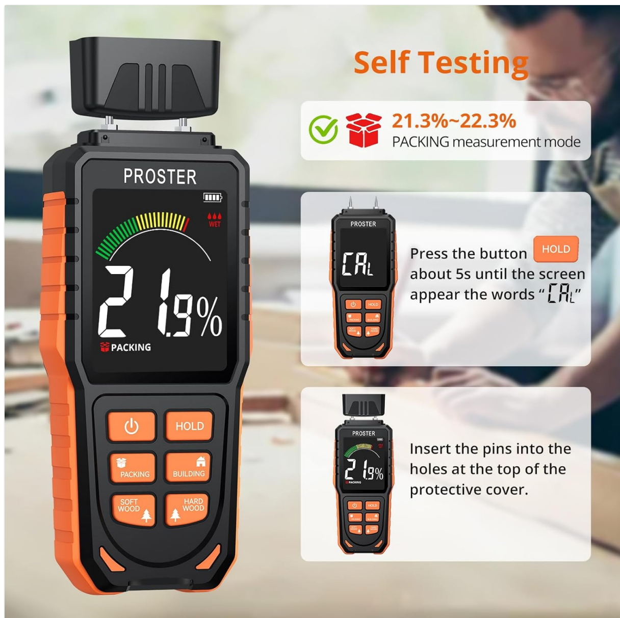
Figure 4: Performing Self-Test Calibration
