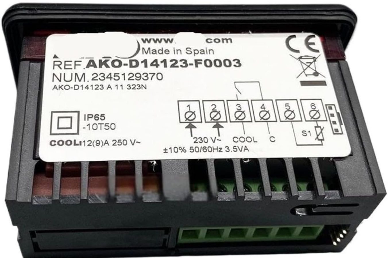
Figure 4: The rear of the controller, displaying the wiring terminals and the product label. The label indicates the model number AKO-D14123-F0003, electrical specifications (230V~, 50/60Hz, 3.5VA), and IP65 rating.
