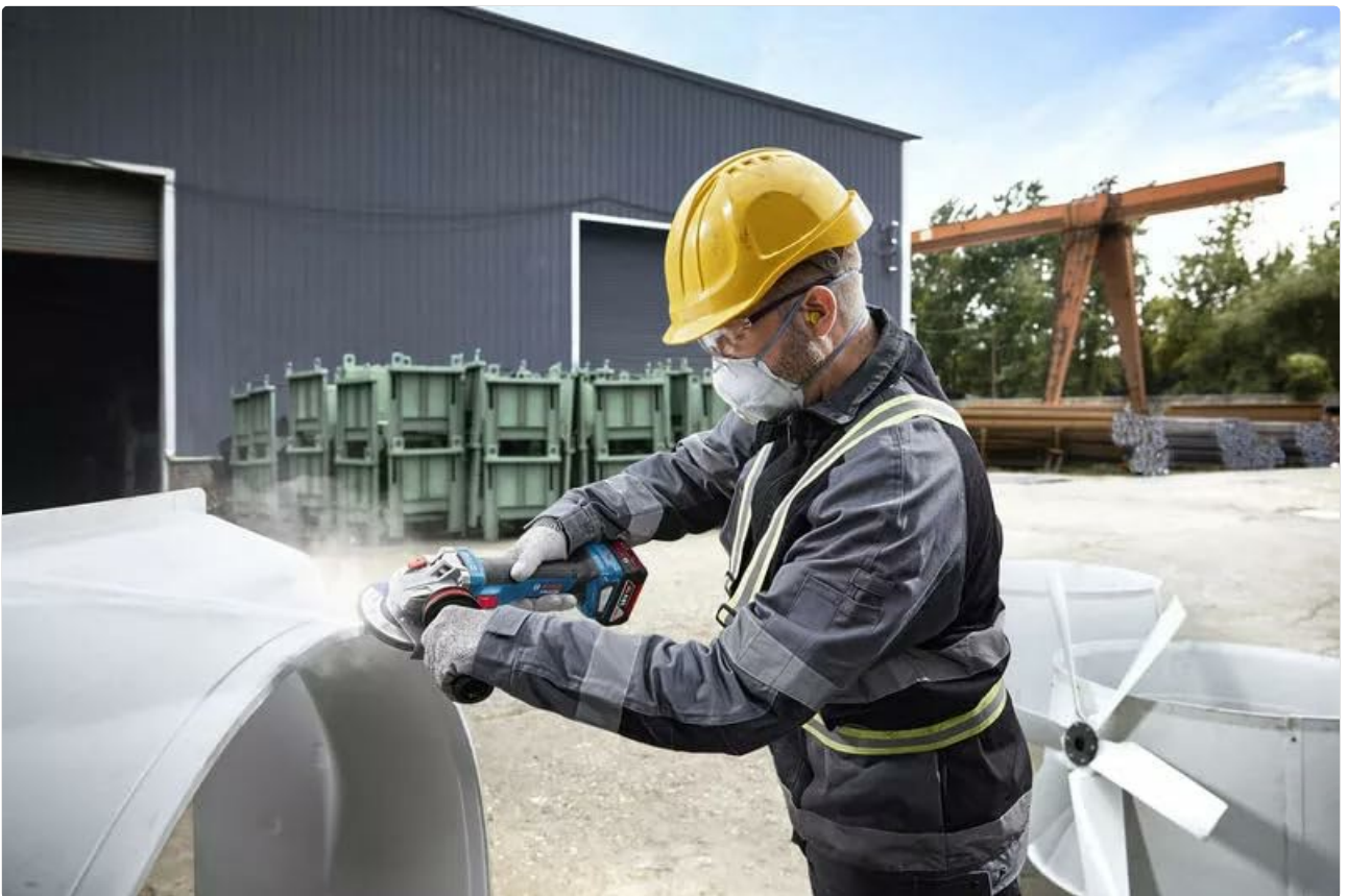
Image: A worker wearing a hard hat and respirator mask using the BOSCH GWS 18V-11 S angle grinder to smooth or deburr a large, curved white surface, creating dust.
