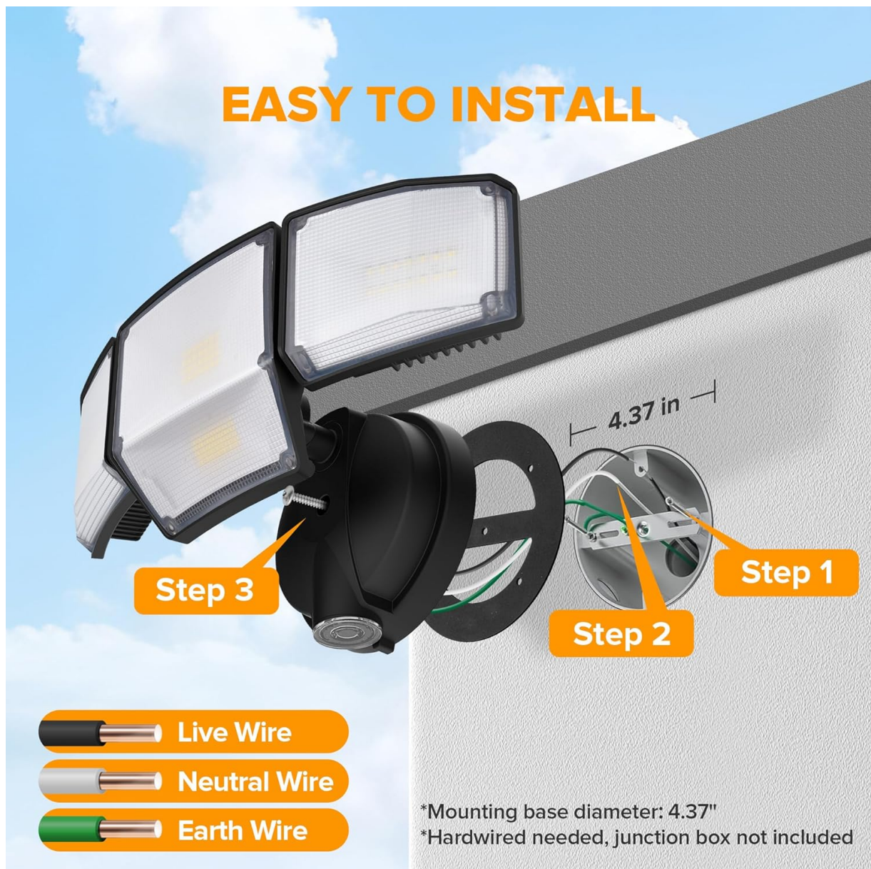
Image 5.1: Hardwired Installation Steps
