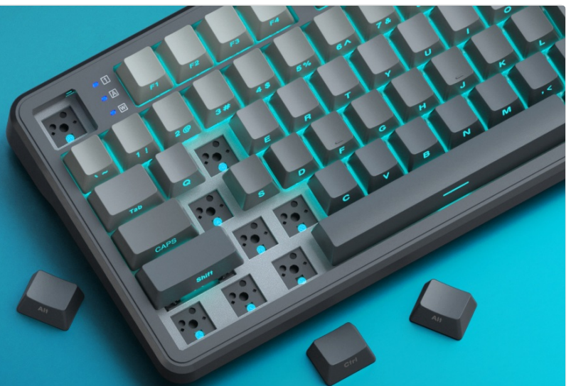
Image: A banner visually demonstrating the hot-swap switch feature of the AULA F108 PRO, showing keycaps and switches removed
